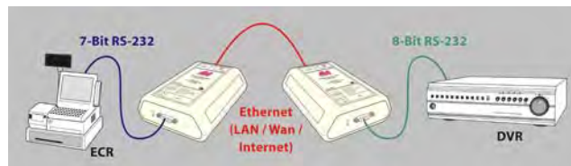
Figure 11: LAVA Ether-Serial Link as serial data formatter
