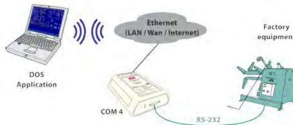
Figure 7: LAVA Ether-Serial Link: DOS interface to factory equipment
