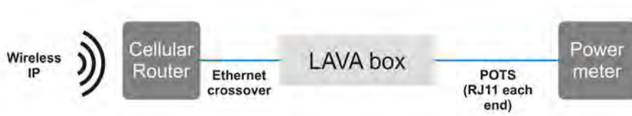
Figure 12: Ether-Serial Link bridging power meter and cellular router
