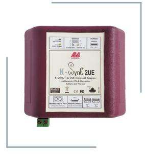
peripherals. When the signal stops, the mobile device will switch into a charge-only mode (default) to recharge the battery.
