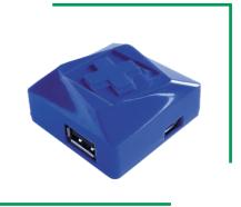
CABM protects the mobile device from overcharging and its battery from bloating, which can cause severe damage. The plug-and-play technology monitors the mobile device as it charges and when the current slows, indicating the device is near a full charge, the adapter disconnects charging power to the mobile device. After a preset number of hours, the mobile device will begin to charge again.
